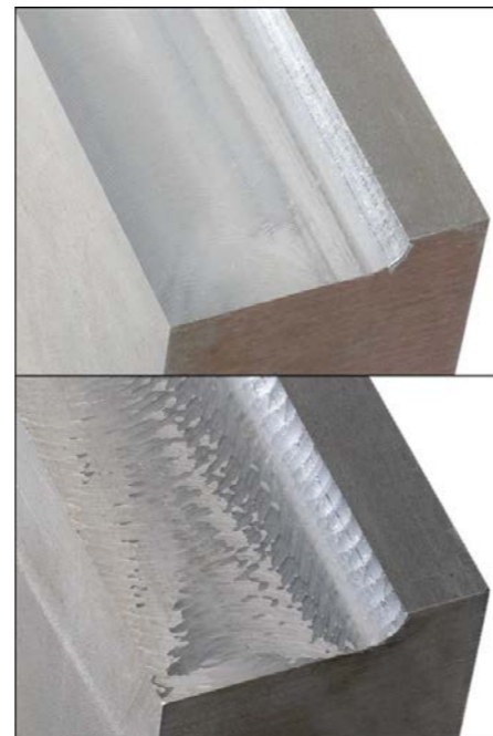
Top figure: part milled with ACC Bottom figure: part milled without ACC
