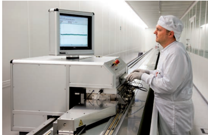
30 m long measuring machine for scale tapes
