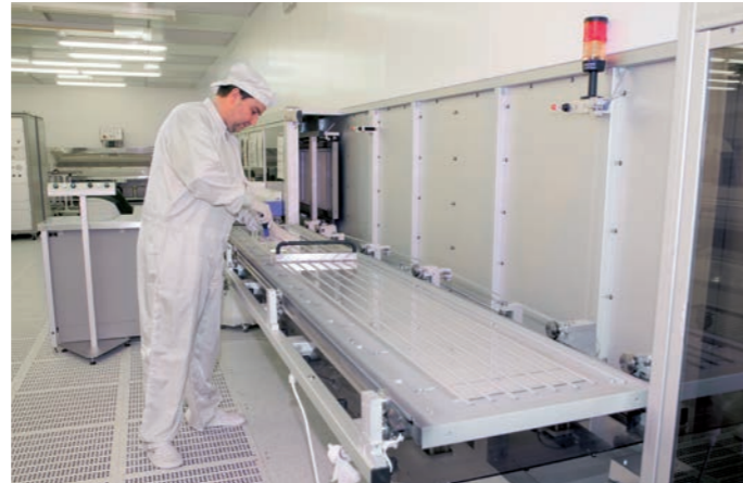
Vacuum machine for application of chromium layers
